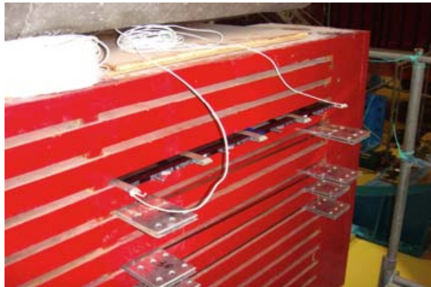
Light yield with cosmic at center of (870mm long) counter
