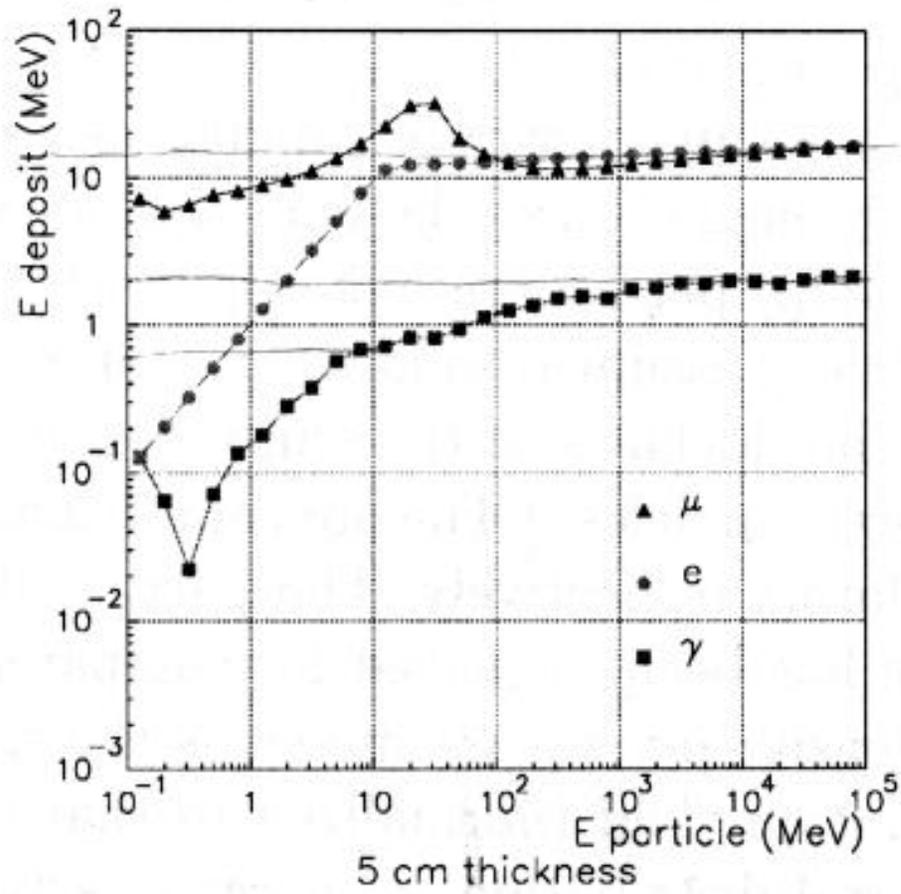
Fig. 1: Average energy deposition arrays for 5 cm thin scintillator. <sup>b</sup>
