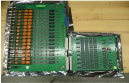
Custom Front-End Electronics Pick-off circuits and discriminators.
