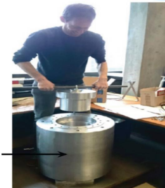
*The largest tungsten compound shielding in the world. The cylinder is 60 cm high and 60 cm in diameter. Thickness is 19 cm. Weight is 2.3 tons. The dimensions are determined by  $^{144}\text{Pr}$  gamma-line with an energy of 2.185 keV (BR = 0.7%), which must be suppressed  $10^{12}$  times and by the size of the hole (1 m) under Borexino. The expected temperature inside is 500 °C, on the surface 80 °C.*
