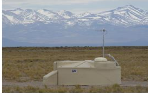
One of the 1 660 water-Cherenkov detectors (WCD) of the Pierre Auger Observatory, located near Malargüe, Argentina (69.3° W, 35.3° S, 9.5 GV) at 1400 m a.s.l.
